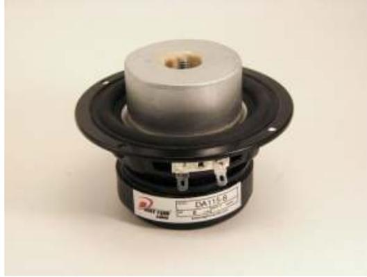
**Figure 15:** Dayton DA115-8 4" linear alternator with the balsa plunger joined to the cone.
