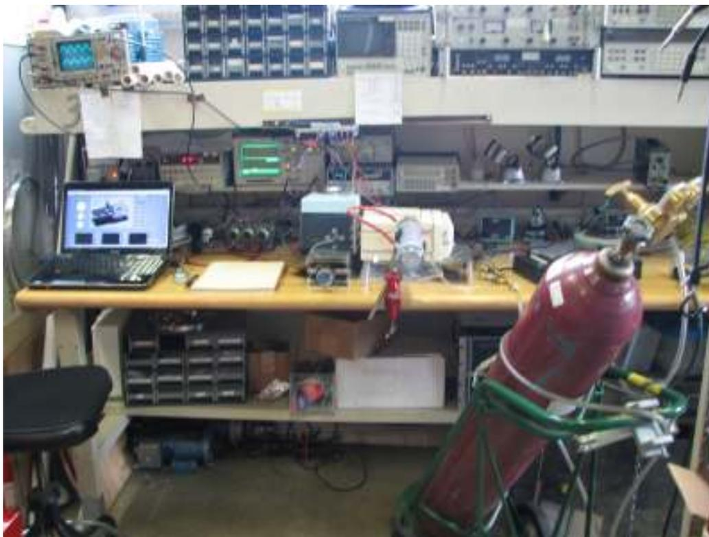
**Figure 20:** Overview of entire lab bench setup while testing was in progress. The data acquisition (laptop) computer is visible at the left. In the right foreground is a cylinder of compressed helium gas that provides a steady stream of gas to improve heat transfer to the hot duct and reduce the oxidation of the NiCr heater element.
