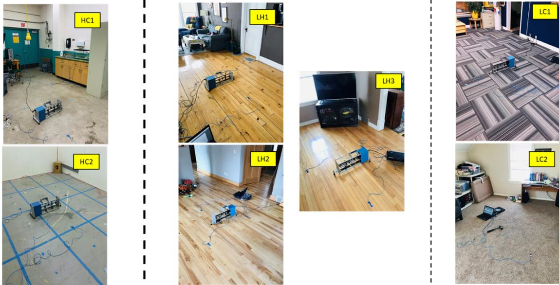
Figure 3-5 Seven floors were tested for the input force measurement with the tapping machine, an impact ball, and the modal hammer: Two heavyweight concrete (HC) floors (left), three lightweight joist-framed floors with hardwood finish (LH) (center), and two lightweight joist-framed floors with carpet finish (LC) (right)
