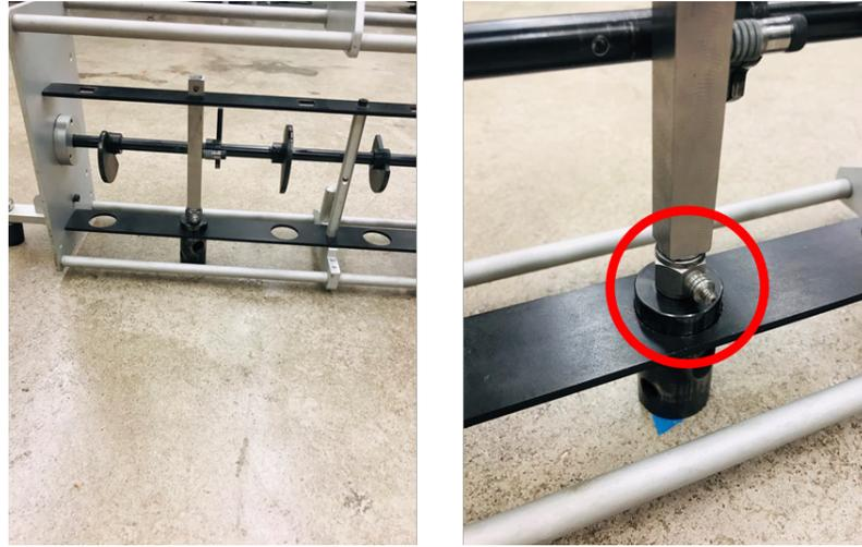
Figure 3-1 Four of the five hammers were removed for simplicity from a standard tapping machine (left) and a force transducer was added between the hammer head and the shaft of the fifth hammer to measure the input force (right)
