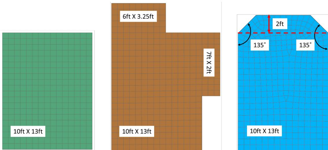
Figure 3-7 The top view of the rectangular shape (left), Coupled Space (CS) assembly with two coupled spaces (center) and a Bay Window (BW) shaped assembly (right) used in the simulation model. For ease of modeling, only concrete assembly was created with the BW shape.
