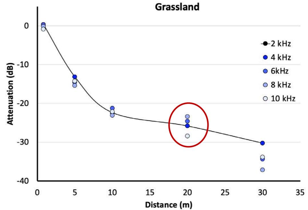
Frequencies between 5-8 kHz cannot be accurately measured in grassland due to singing insects
